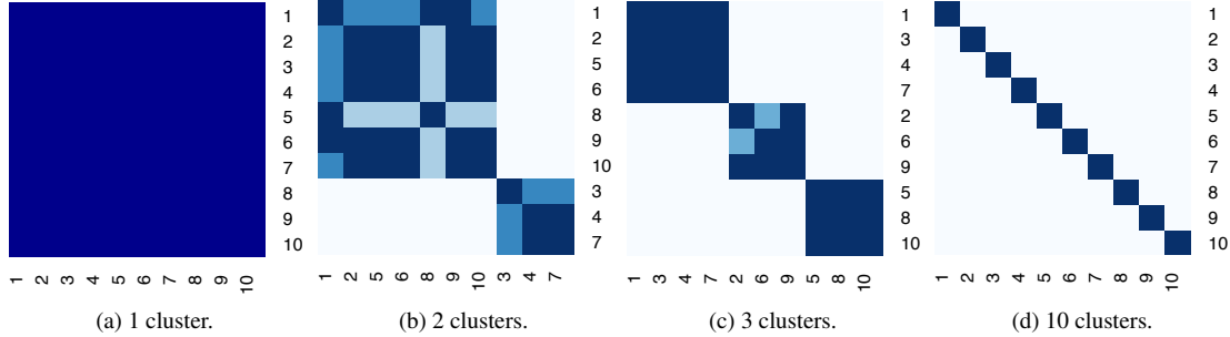
Fig. 3: Heatmap (or classification matrix) describing the efficiency of our clustering algorithm with n around 300, see Table 3. Values for the percentage of right predictions are given from very light to dark blue, which corresponds to no error (0%), [80%, 90%[, [90%, 100%[, 100%
